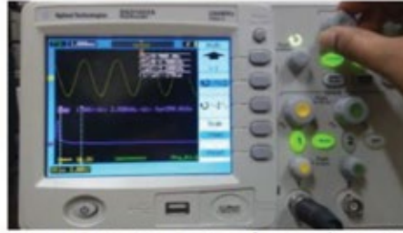
Viewing Fast Fourier Transform on the DSO
